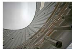
Advanced Materials: Carbon fiber in the fuselage (see photo) along with other composites and advanced alloys are being used to increase strength and reduce overall weight of an aircraft.
